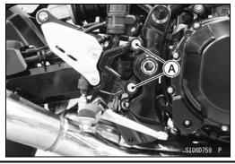
• Install the bracket [4] and tighten the bolts [5].
