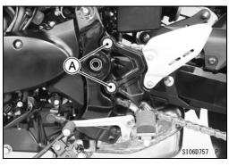
• Remove the right front footpeg bracket bolts [A].
