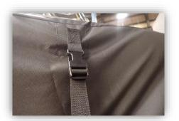
• Pull cover down around rear wheels. Clip lower rear straps together and tighten.
