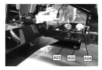
6. Position spacer 2 (A06) between the hitch bracket (A01) and hitch support bracket (A02). Secure with two (2) M12 flange hex screws (A03) and two (2) M12 flange nuts (A04).
