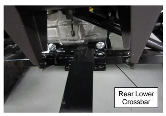
4. While holding the hitch bracket (A01) in place, assemble the hitch support bracket (A02) behind and underneath the rear lower crossbar as shown.
