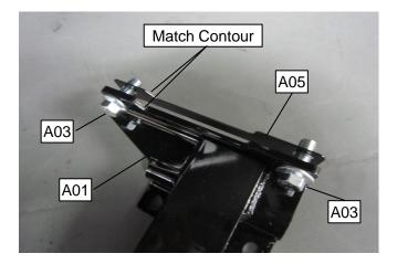
3. Center the partially assembled hitch bracket onto the rear lower crossbar as shown.
