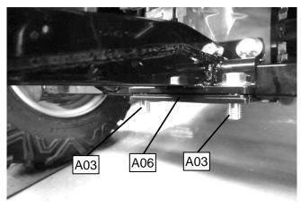
7. Tighten all hardware in the number sequence shown by tightening all hardware to the initial torque value, then tightening to the final torque value.
