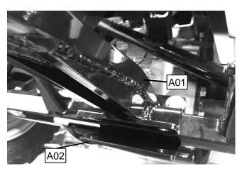
5. Slide the hitch support bracket (A02) rear hole through the two (2) M12 flange hex screw (A03) and loosely install the two (2) M12 flange nuts (A04).
