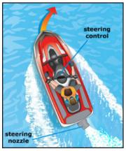
The most important thing to remember about steering is that you must have power to turn. If you release the throttle or shut off the engine, the craft will lose the very force that enables its steering. Some PWC today have throttle reapplication devices to assist steering if you release the throttle, however, you should assume that you will need throttle to steer.
